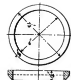
Figs. 239-240. Ground Washer for Dry Pipe Ball Joint.
